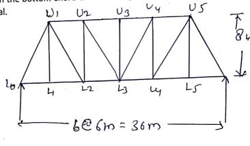
Q. 9 Draw ILD for forces in member due to  $U_2U_3$ ,  $L_2L_3$  and  $U_1L_1$  of a pratt truss as shown in fig. 2.
